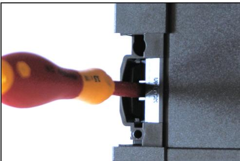
We recommend to unlock at least 2 snap-in pins at the same time. When removing carefully the upper part of the enclosure ensure that front plate and rear plate remain in the lower part of the enclosure!
